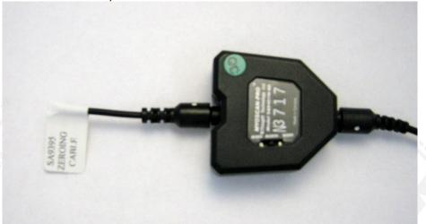
With the zeroing plug on the sensor, the reading should be zero. If your software displays a different value, usually plus or minus a few microvolts, then you should be able to correct this offset, from within the software, by using a zeroing function. Keep in mind that each sensor may have different offset values, and that the offset may change, particularly with temperature. **Remember to remove the zeroing plug after adjusting the MyoScan-Pro sensor's offset.**
